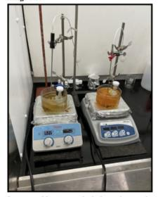
Storing and heating methods for vials at each temperature Image 1.4:
